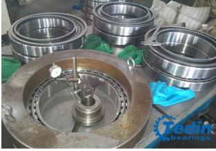
Single row tapered roller bearings can support axial forces in one direction and high radial forces. If the load carrying capacity of one bearing is not sufficient or the shaft is to be guided with a certain axial clearance in both directions, matched pair tapered roller bearings are available.
